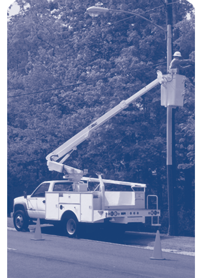
(b) Telescopic aerial device. (Fig. 2/ Telescopic Aerial/Device (Bucket Truck)/Used with permission of Altec Industries)
