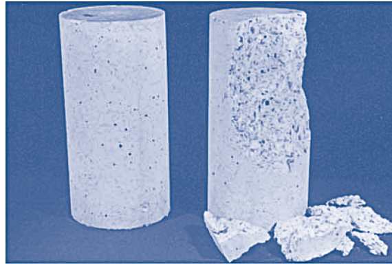
(c) A concrete cylinder before and after compression testing. (Courtesy Roy Craig)
