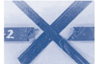
FIGURE 2.19 A graphite-epoxy tensile test specimen; \pm 45^\circ graphite-fiber lamina.
